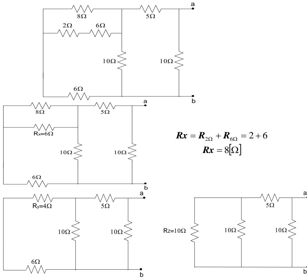
$$\frac{1}{R_y} = \left[ \frac{1}{R_x} + \frac{1}{R_{8\Omega}} \right] = \frac{1}{8} + \frac{1}{8}$$
