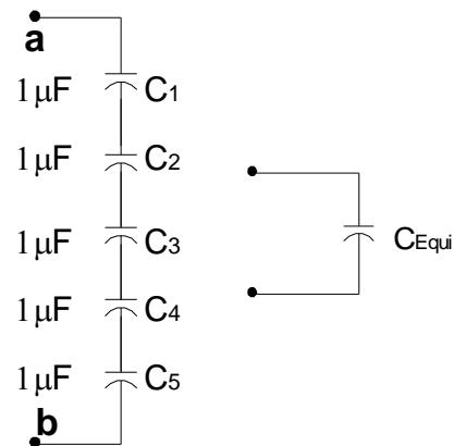
$$\frac{1}{C_{Equi}} = \frac{1}{C_1} + \frac{1}{C_2} + \frac{1}{C_3} + \frac{1}{C_4} + \frac{1}{C_5}$$
