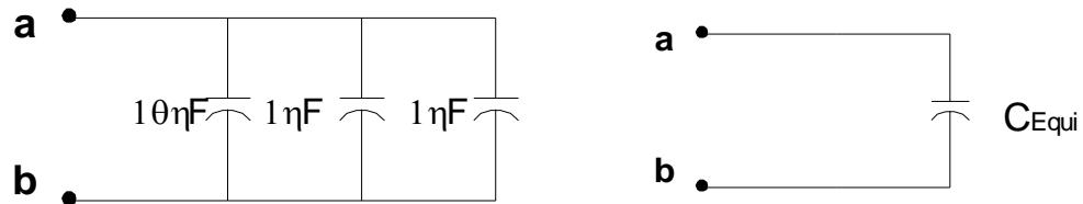
$$C_{Equi.} = C_1 + C_2 + C_3$$
